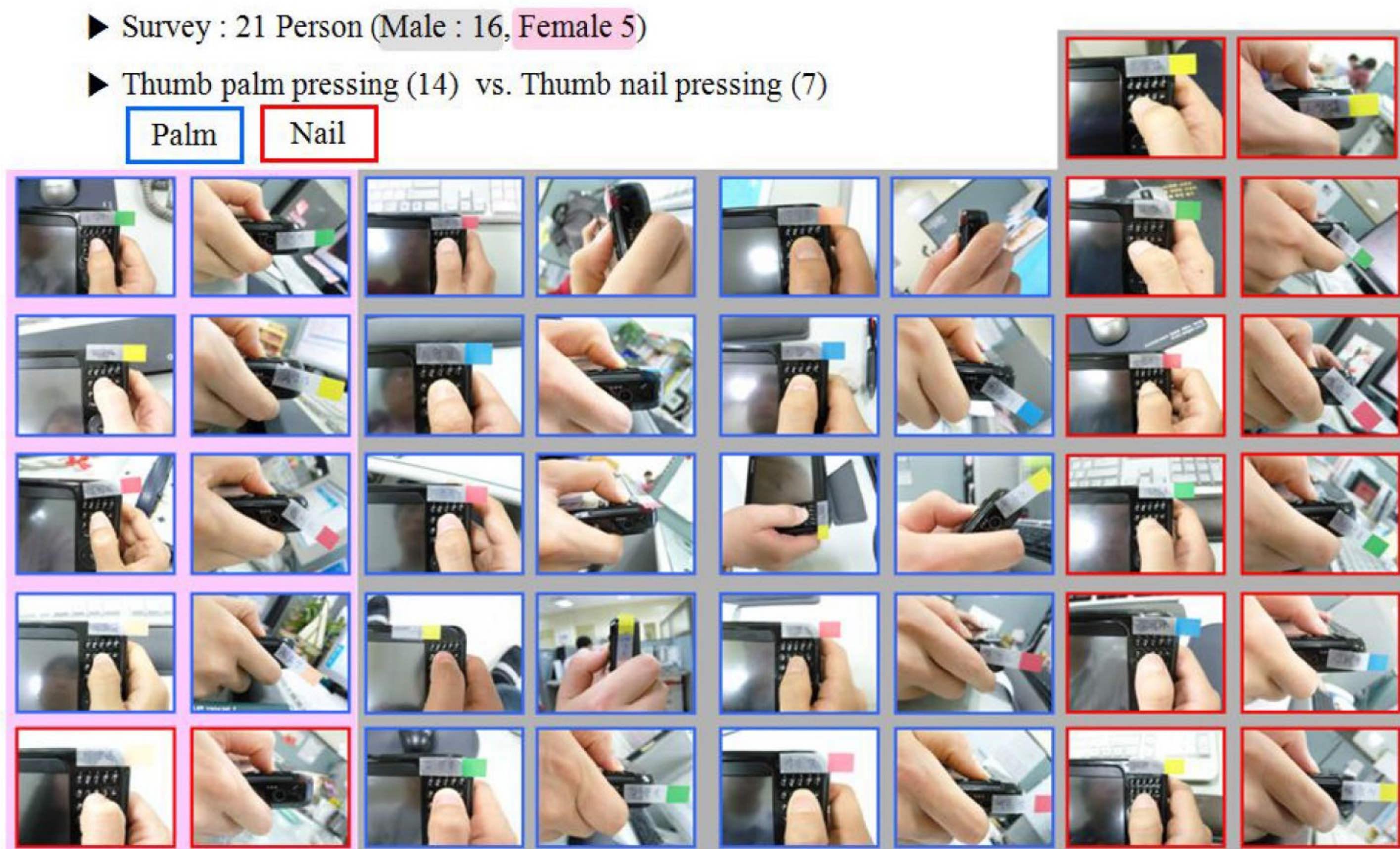
Image 3. To study thumb-strike angle variety, 21 volunteers from the Samsung research facility were photographed as they worked the keypad of the prototype device.
