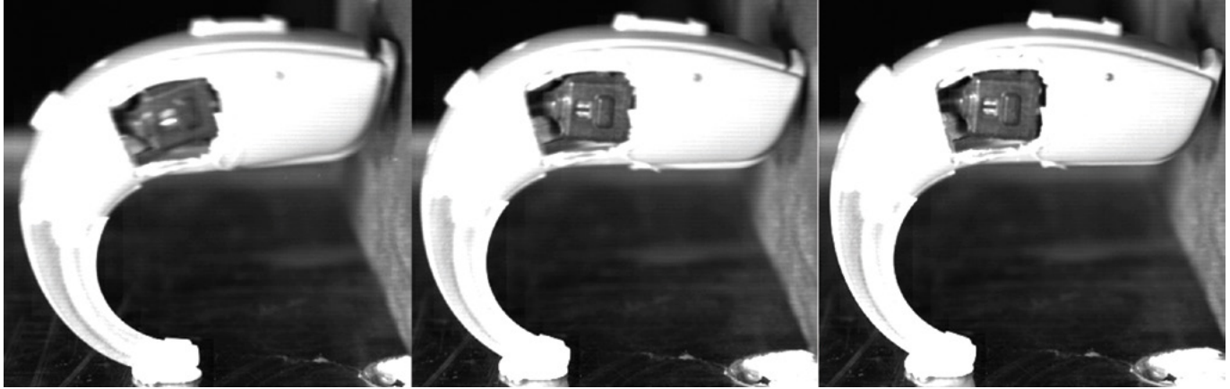
Image 4. High-speed video is used to record impact. Left photo is 0.9 after impact, middle is 0.1 after impact, right is at impact. Note motion of receiver at center of device.
